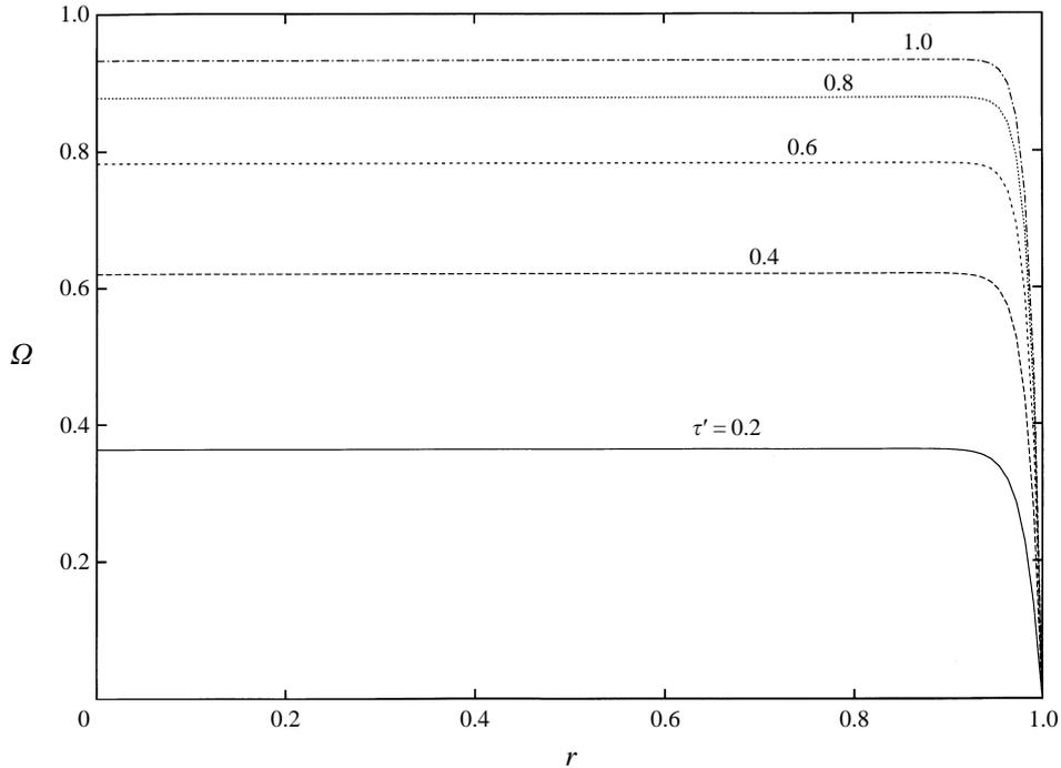
FIGURE 2.  $\Omega$  vs.  $r$  (in core and near sidewall), for various  $\tau'$  ( $= \tau\kappa$ ), upper and lower walls rigid,  $(HE^{1/2}/\kappa) = 10^{-2}$ . Spin-up from rest
